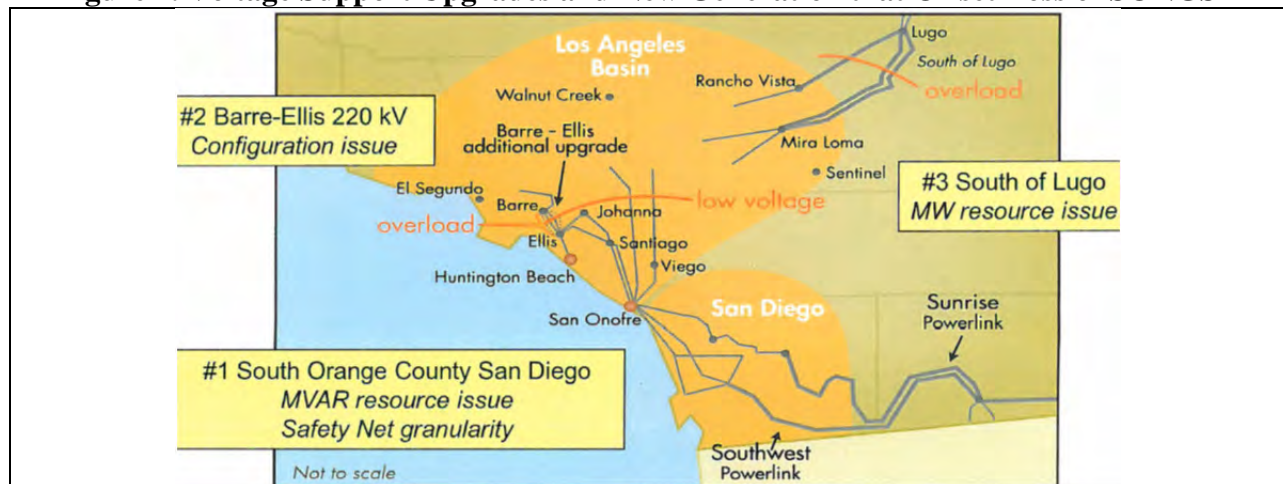
Figure 7. Voltage Support Upgrades and New Generation that Offset Loss of SONGS 44
