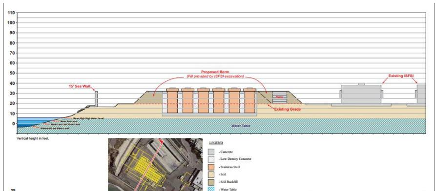
*Side cutaway view of the proposed Holtec ISFSI*
