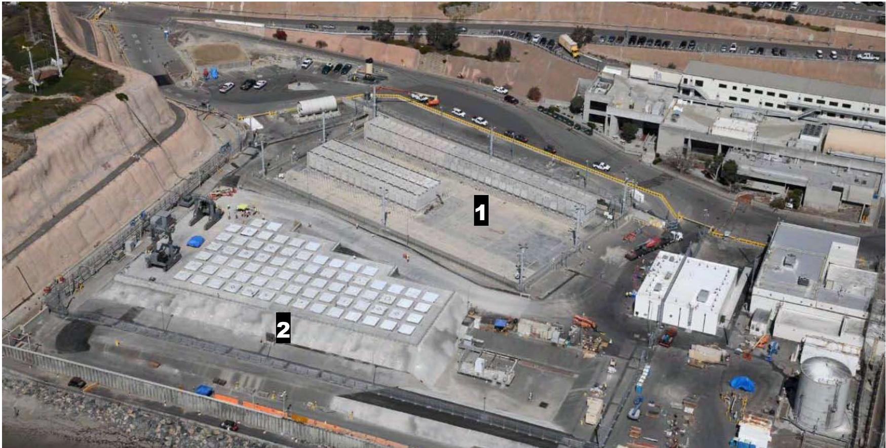
**The storage pad, or Independent Spent Fuel Storage Installation, is located north of the plant. The spent fuel for Unit 1 is housed in horizontal vaults (1). The MPC containing spent fuel for Units 2 and 3 are being placed in underground vaults (2) (each white circle marks an MPC storage location.)**
