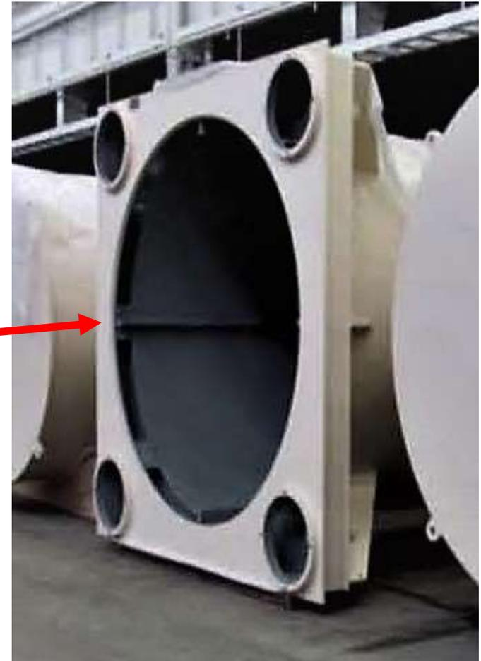
The MPC fits into the CEC like a hand in glove, except in this case the glove is rigidly made from steel. Guide ribs help align the MPC over the CEC and guide its lowering into place.
