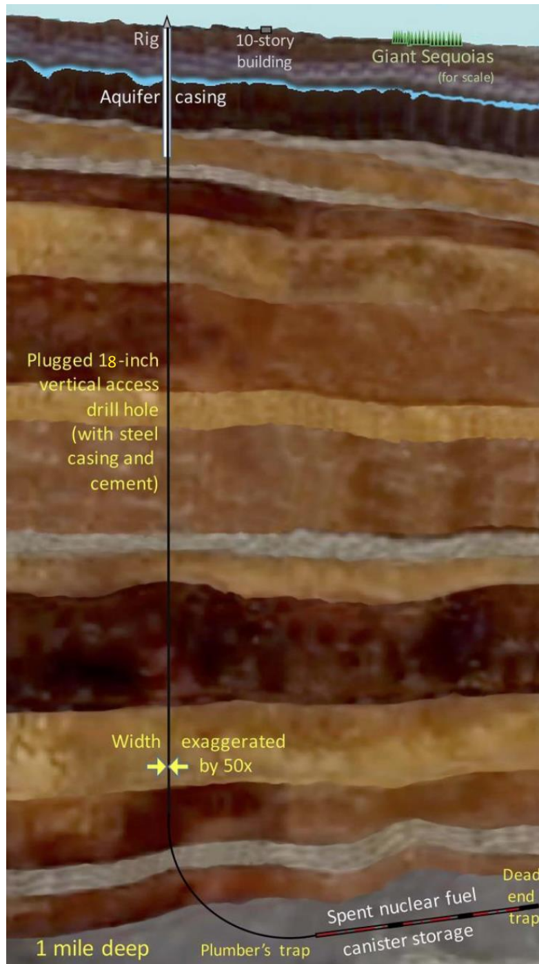
Figure 1. Deep Isolation Repository Baseline Design This diagram shows a relatively short horizontal section; in practice, it could be 1 to 3 km long.
