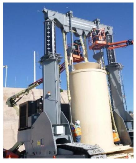
This photo shows the canister ready for downloading, the vertical cask transporter lift beam has been raised, and the full load of the spent fuel canister is being suspended. The mating device door is open, allowing the canister to be downloaded
