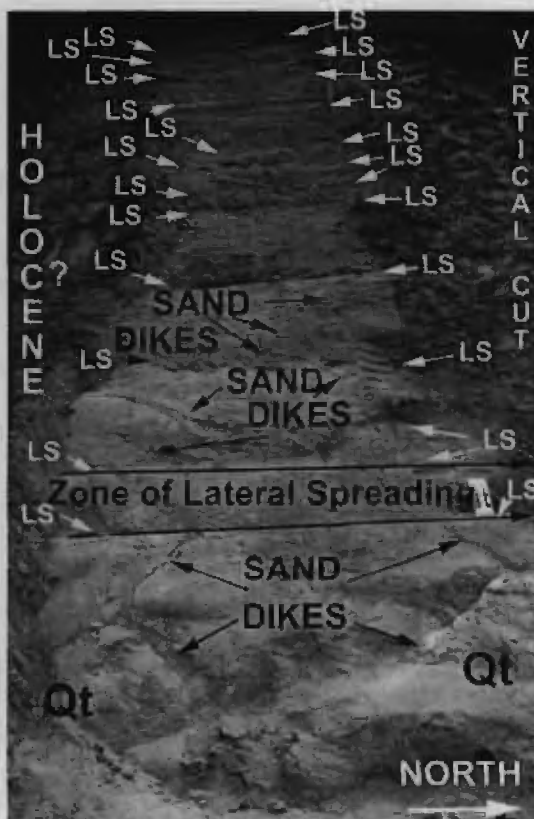
Fig. 25. Photograph of a vertical cut exposing sand dikes cutting coastal terrace sands at Carlsbad, California (47.24–51.81 m el. MSL) Note: The scale is resting on a lateral spread surface that has cut-off the underlying sand dikes, which were injected from below. At least 10 episodes of lateral spreads cut-off sand dikes. Measured sections of multiple lateral spread surfaces in vertical cuts are shown in Fig. 26.
