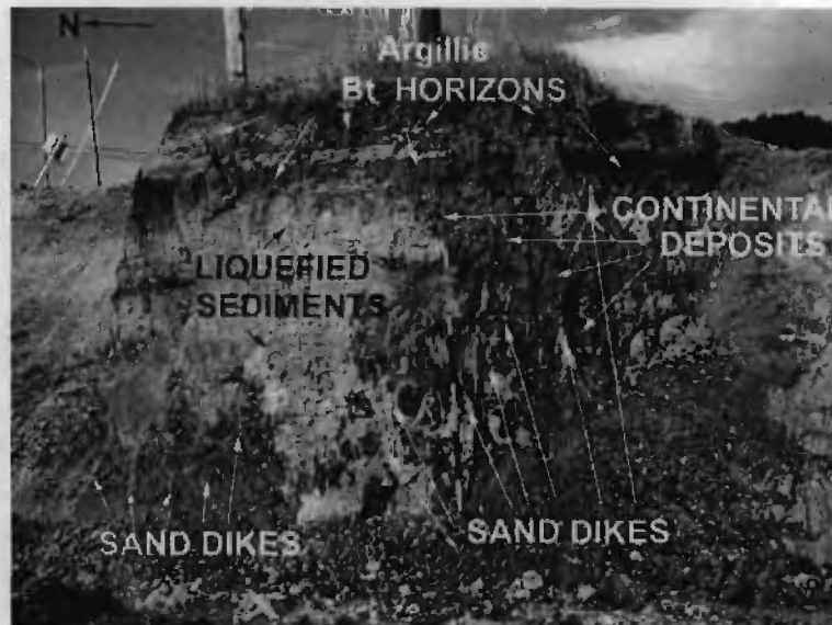
Fig. 6. View (1994) of a railroad cut exposure showing fine grain, tan and white sand dikes cutting into and through continental deposits and into an overlying Bt argillie soil horizon at Carlsbad, California (15.24 m el. MSL).
