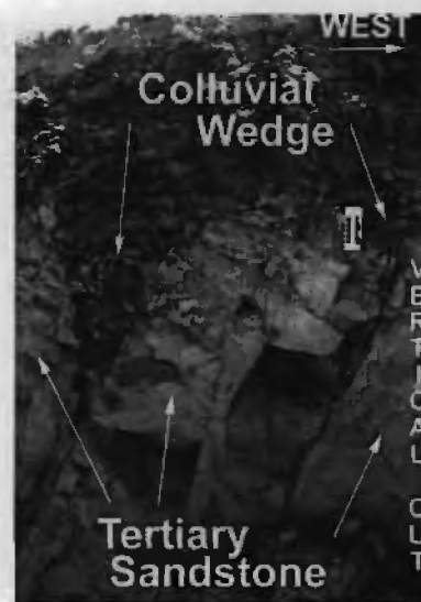
Fig. 24. Colluvial wedges; inferred to be large fissure fills exposed in Tertiary sandstone (fractured grey-white unit) at Carlsbad, California (6.09–7.62 m el. MSL).
