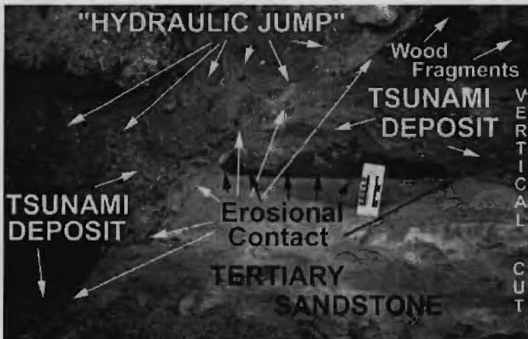
Fig. 34. North wall of a sewer-line trench cut into a terrace and exposing a possible paleotsunami deposit at Encinitas, California (93.26 m el. MSL). Note: The scale is located on a Tertiary-age sandstone abrasion platform, which is unconformably capped by a chaotic, turbid deposit containing small angular pieces of terrace and “parent” Tertiary sandstone and small rocks. Also note the “v-shaped upward climbing” chaotic features interpreted to result from an abrupt “hydraulic jump” created when tsunami waves reached a bedrock high.
