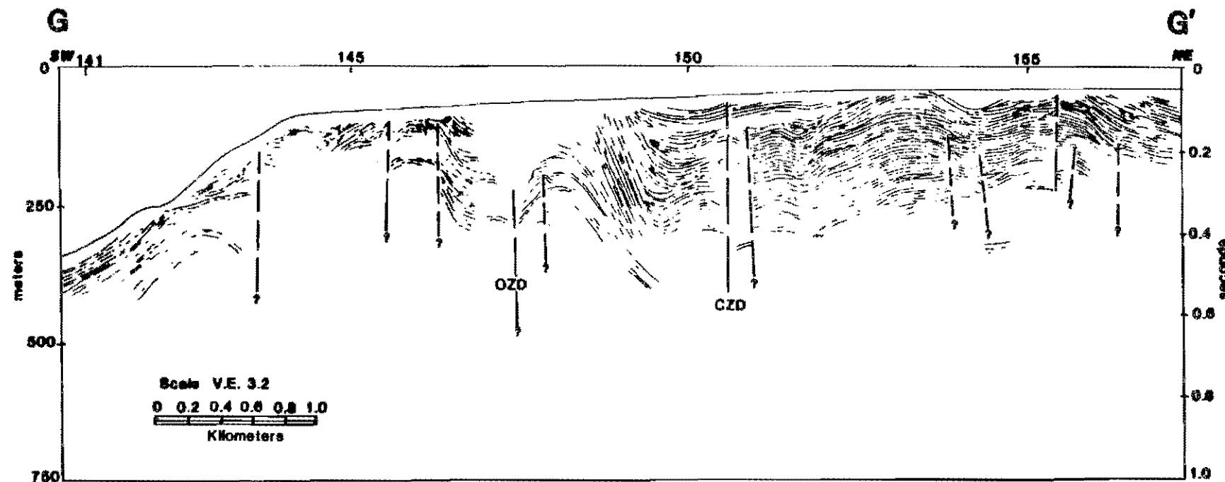
Figure 7.--Line drawing of Marine Advisor's seismic reflection profile S-16 showing OZD, CZD, and other structure in study area. See Plates 1 and 2 for location.
