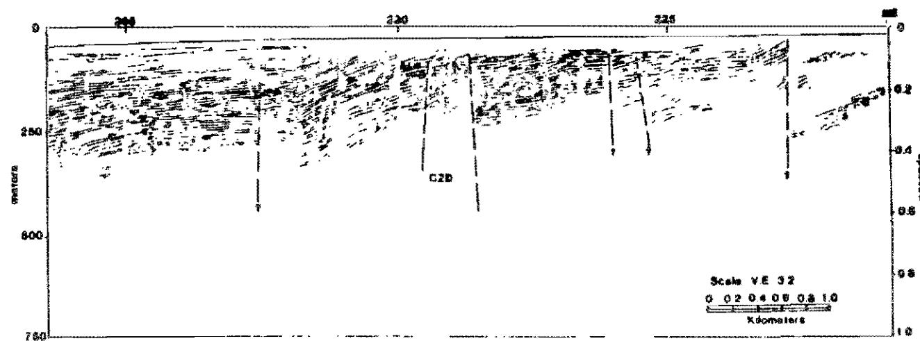
Figure 1.--Line drawing Marine Advisor's seismic reflection profile S-22 showing location of the CZD and CZD. See Plates 1 and 2 for location.
