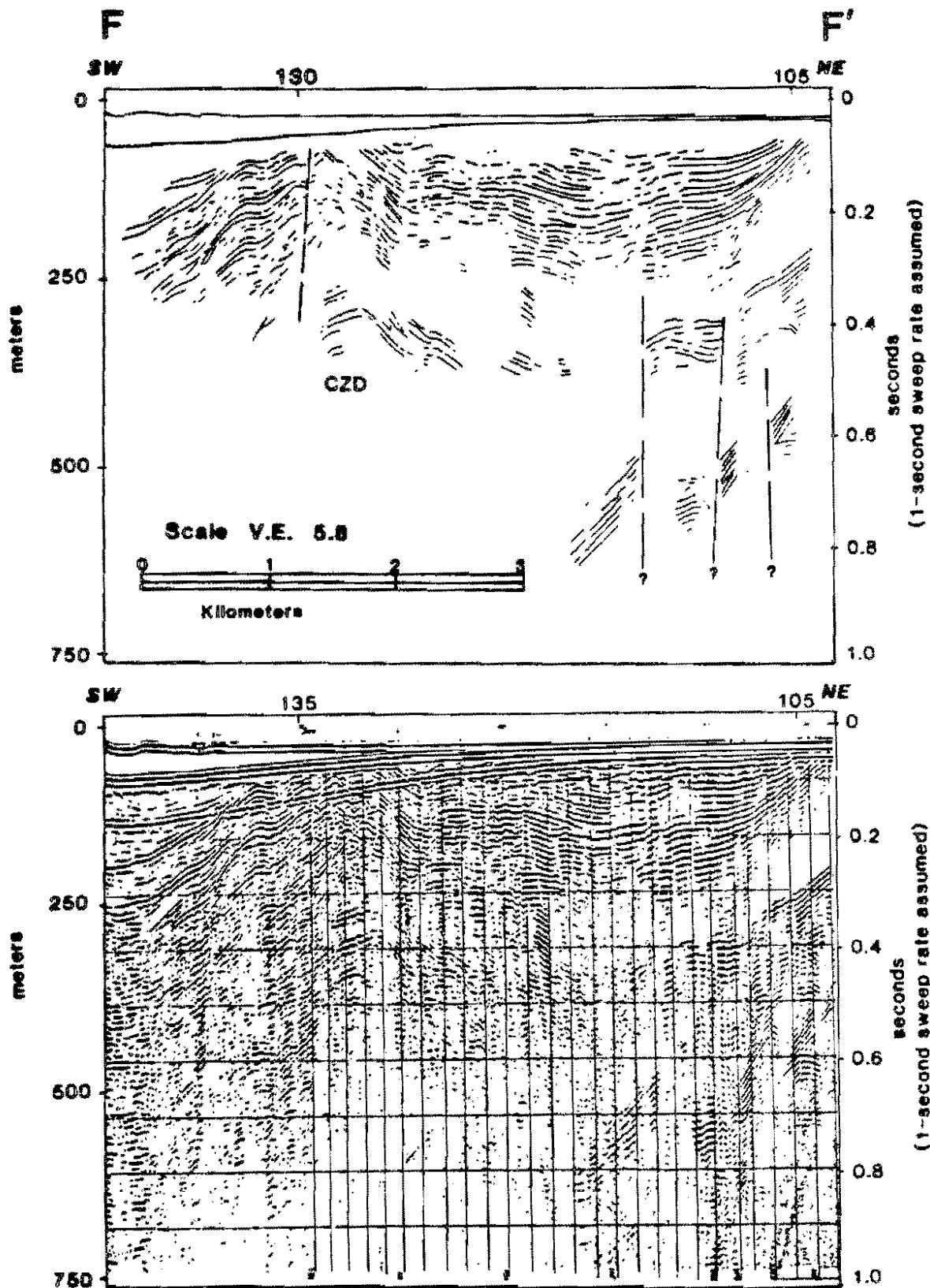
Figure 6.--Line drawing and seismic reflection profile of Woodward-Clyde Consultant's Line B16 showing CZD and deep faults nearshore. See Plates 1 and 2 for location.
