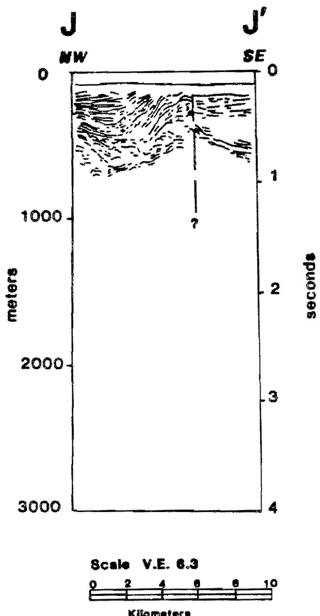
Figure 10.--Line drawing of USGS seismic reflection profile 57 (S2-79-SC) showing fault inshore of CZD. See Plates 1 and 2 for location.
