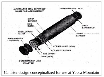
been more merit in a slightly different design by enclosing the drip shield as a second layer and making it part of the cask, similar to the facility provided by the dual-layer MELO design.
