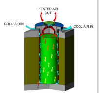
Atmospheric air flows right over the canisters, shown in the belowground Holtec UMAX ISFSI design
