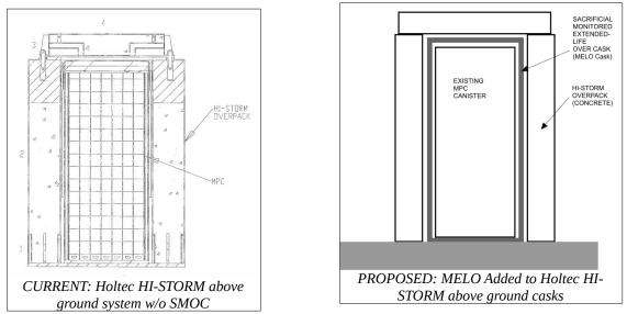
Above-ground systems can add the MELO Cask fairly easily by removing the outer concrete overpack and adding the MELO Cask, and then adding a new, larger concrete overpack.
