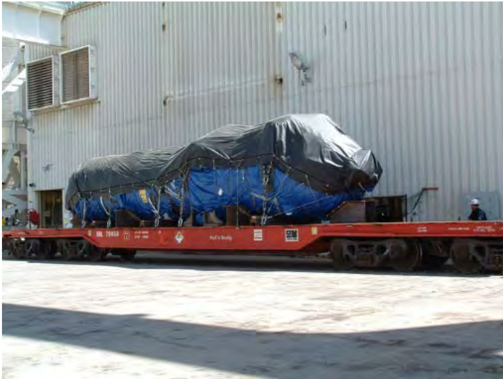
Figure 2-95. Rancho Seco Pressurizer on Railcar (2004)
