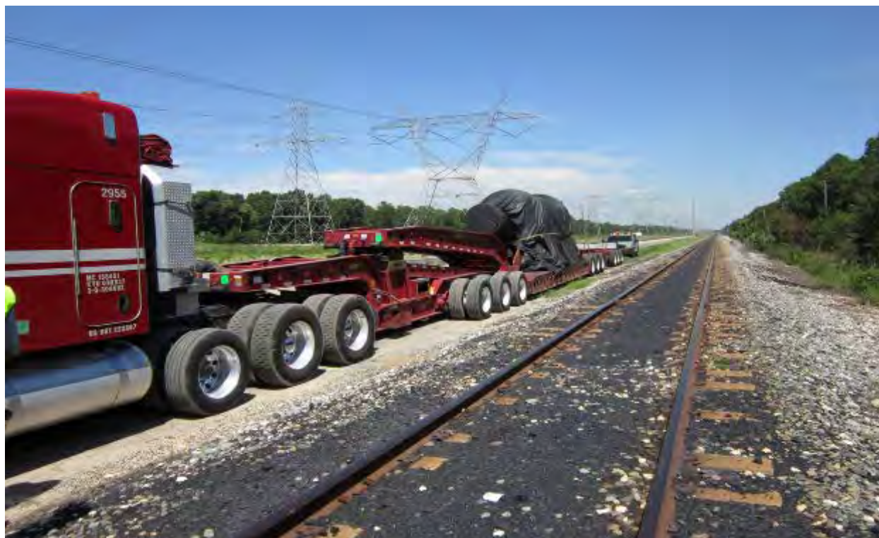
Figure 2-199. High Pressure Turbine Rotor Delivered to Crystal River Site by Heavy Haul Truck (2011)
