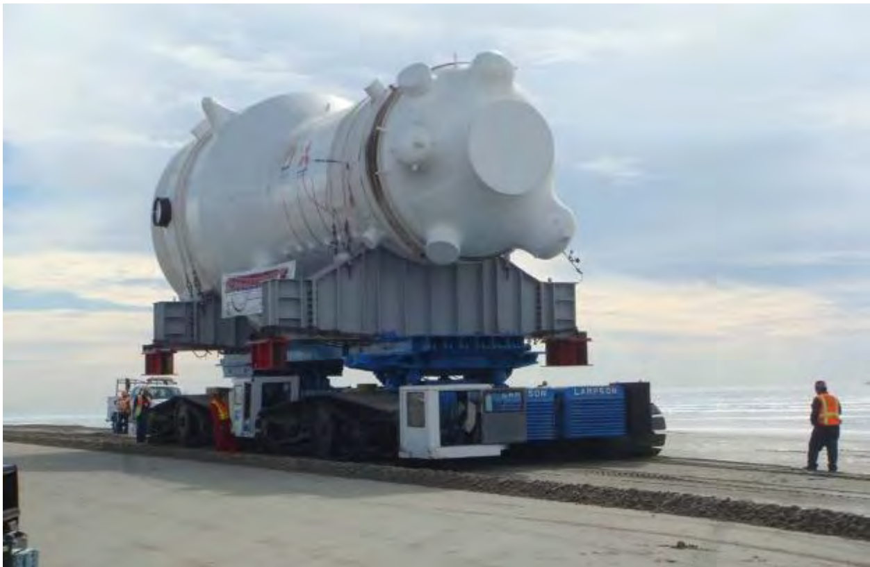
Figure 2-296. Steam Generator on Tracked Vehicle on Beach (2009)
