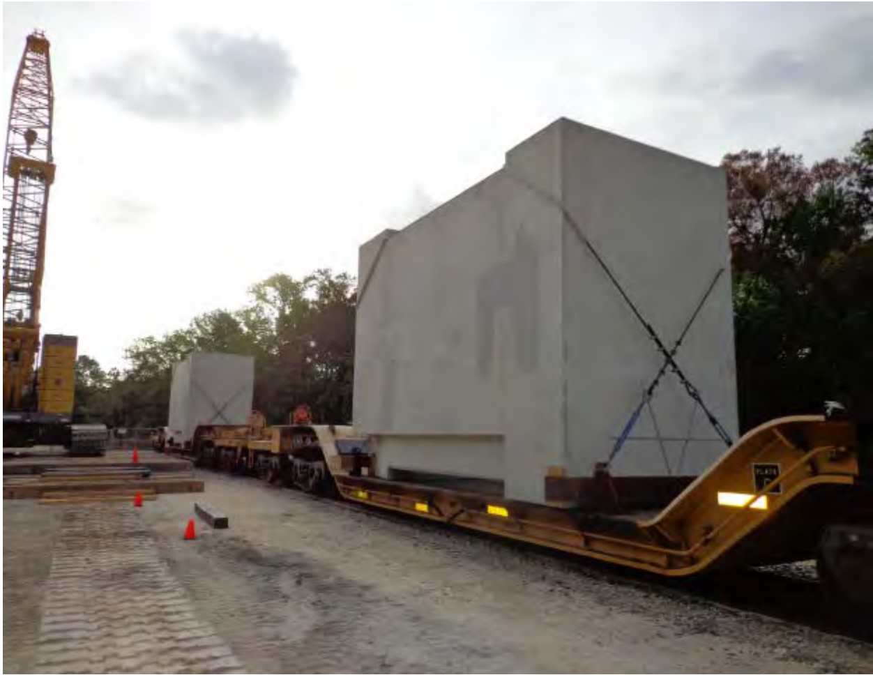
Figure 2-186. Two Horizontal Storage Modules Loaded on Railcars (2015)
