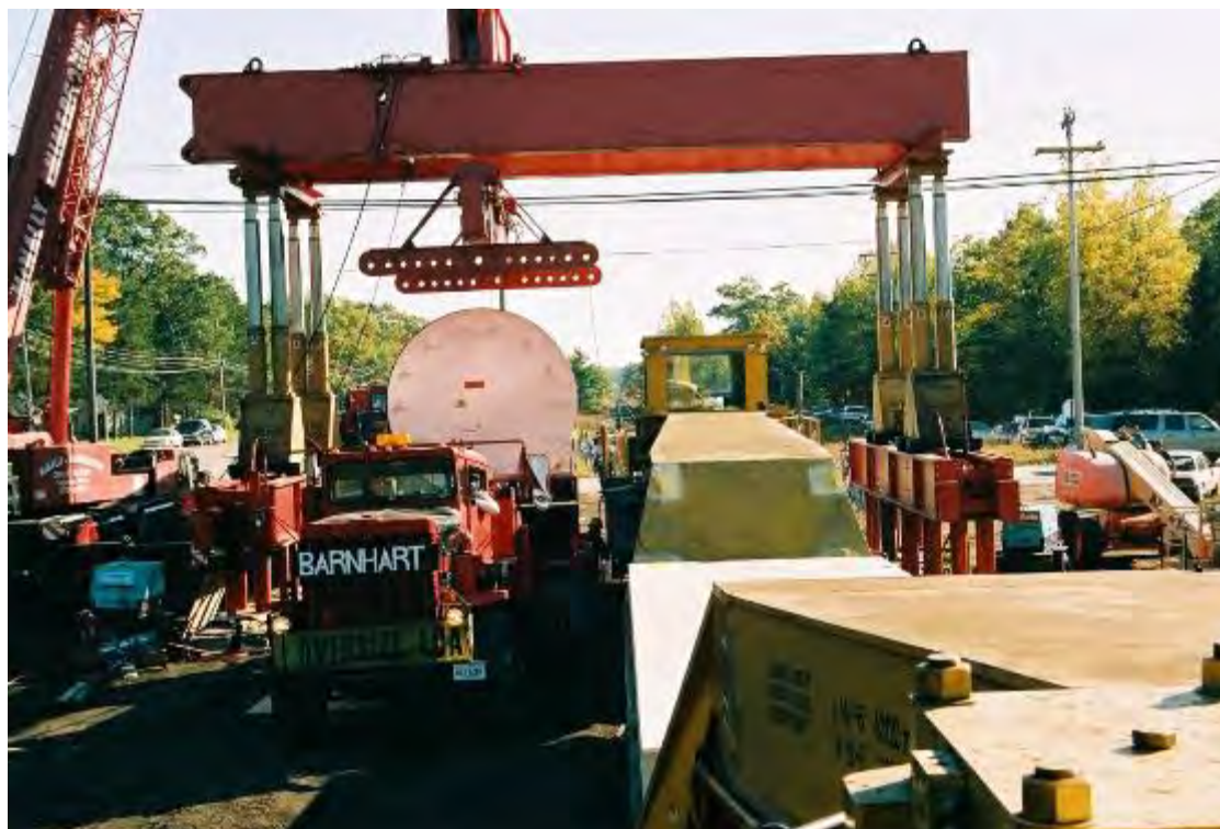
Figure 2-71. Heavy Haul Truck with Reactor Pressure Vessel beside ETMX1001 Railcar (2003)
