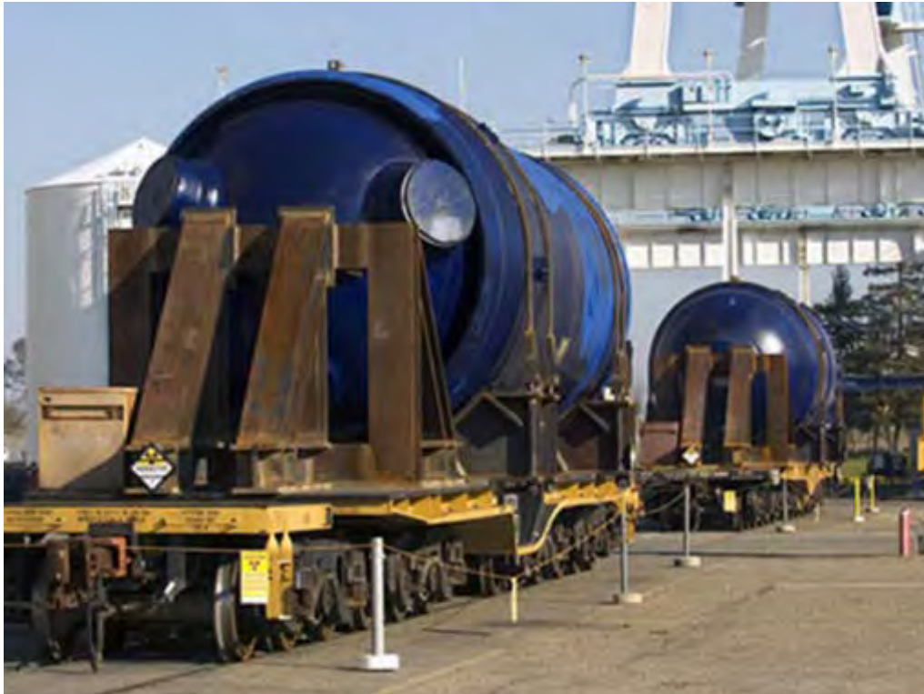
Figure 2-96. Rancho Seco Steam Generator Segments on Railcars
