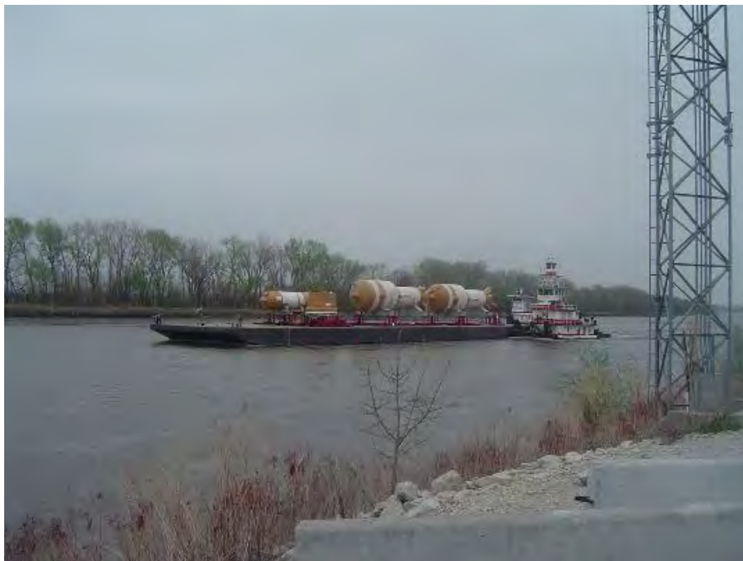
Figure 2-365. Steam Generators, Pressurizer, and Reactor Vessel Head Being Shipped by Barge (2006)
