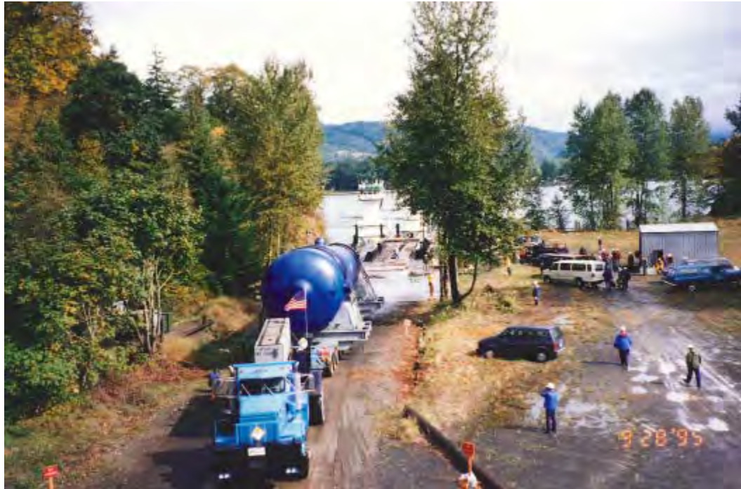
Figure 2-114. Trojan Steam Generator Being Loaded at Barge Slip (1995)
