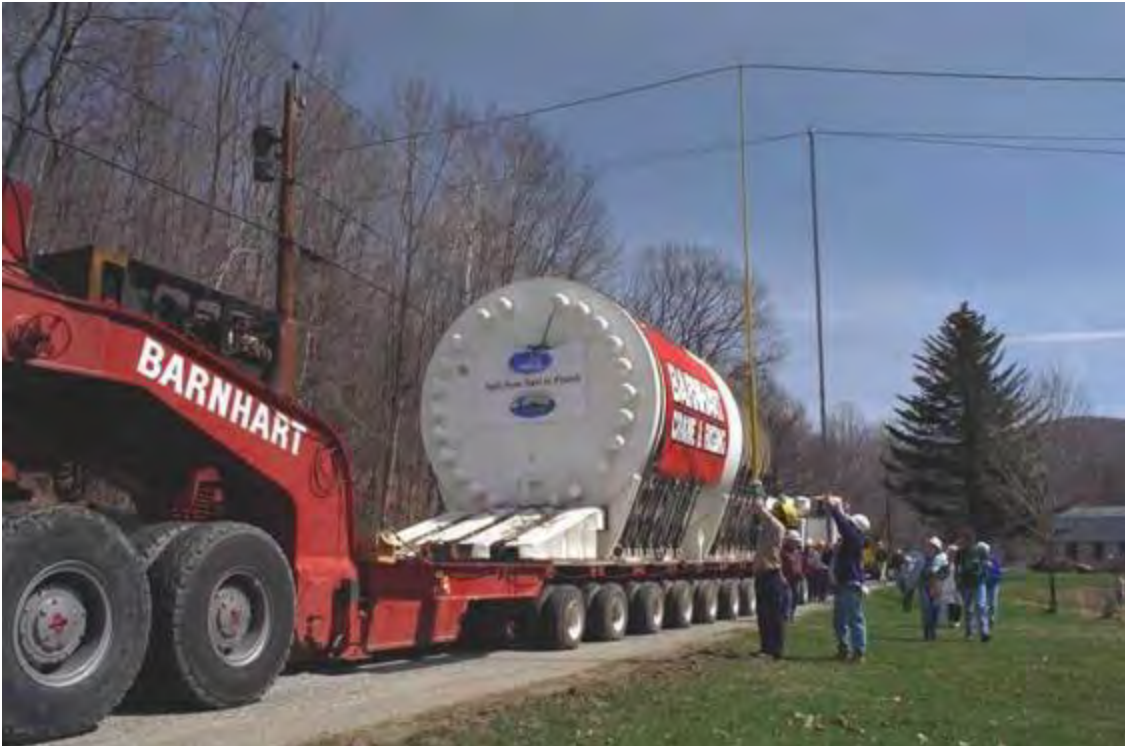
Figure 2-26. Yankee Rowe Reactor Pressure Vessel on Heavy Haul Truck Moving Under Power Lines (1997)
